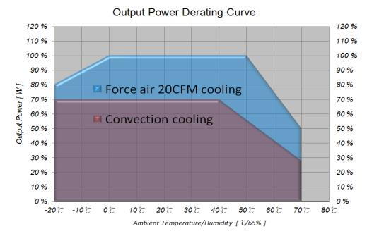
convection cooling Derate linearly 2.5% per °C from 41 to 70°C 20CFM forced air cooling Derate linearly 2.5% per °C from 51 to 70°C 20CFM forced air cooling Derate linearly 1.0% per °C from 0 to -20°C
